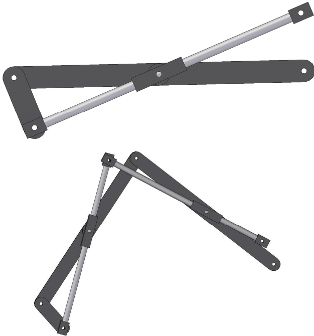
Fig. 4. Primary and secondary 3 bar slider-pivot linkages
